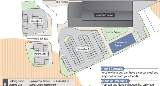
Building use Store, Office, Restaurant Structure & size Structure Steel construction One-story Size 297 14 m<sup>2</sup> Building area Total floor space 296.98 m<sup>2</sup> Maximum height 5.09 m
